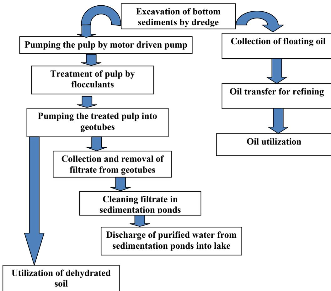
**Fig. 1.** Technological scheme for remediation of bottom sediments of three lakes polluted with oil.
